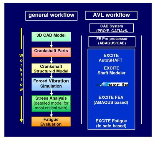
Fig. 7. Workflow for durability of crankshafts (structured model)
