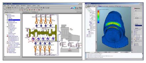
Fig. 6. System modelling and result evaluation for engine durability simulation
