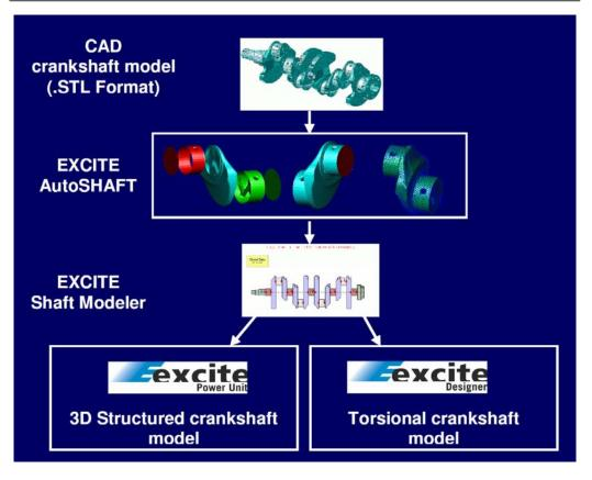
Fig. 8. Flexible crankshaft MBS model for 1D and 3D analysis automated derived from CAD-STL file
