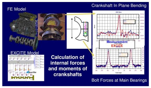
Fig. 9. Comparison of results for a crankshaft of a 4-cylinder engine
